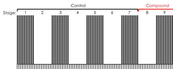
**Figure 1: Modified Milnes protocol.** The Milnes protocol consists of 9 stages, each 250 seconds long. Depolarising stages (1,3,5,7,9) consist of 10 depolarisations for 10 seconds each with a sweep-to-sweep interval of 25 seconds. A single concentration of compound is applied during stages 8 and 9.
